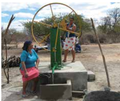
Figure 4 A manual water pump provides water for animals
